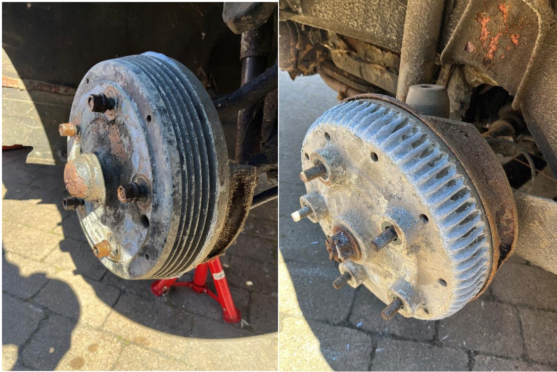
Above GT brakes (left), and ventilated backing plates in the rear brakes (right)
