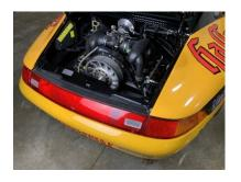
were powder coated. Factory motorsport headers retained. Single O2 sensor catalytic converter was cut open to remove clogged cats and rewelded to retain the factory look. Non-original exhaust tips were replaced with reproductions made to match the factory cup pieces which are NLA. All the factory heat shielding is in place and correct for the 993 cup. New fuel filter and fuel pump.
